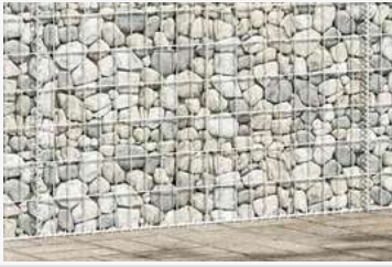
Gabion plein concassé calcaire beige, dim.L100xI50xH50cm, dim. fil 5.8mm
